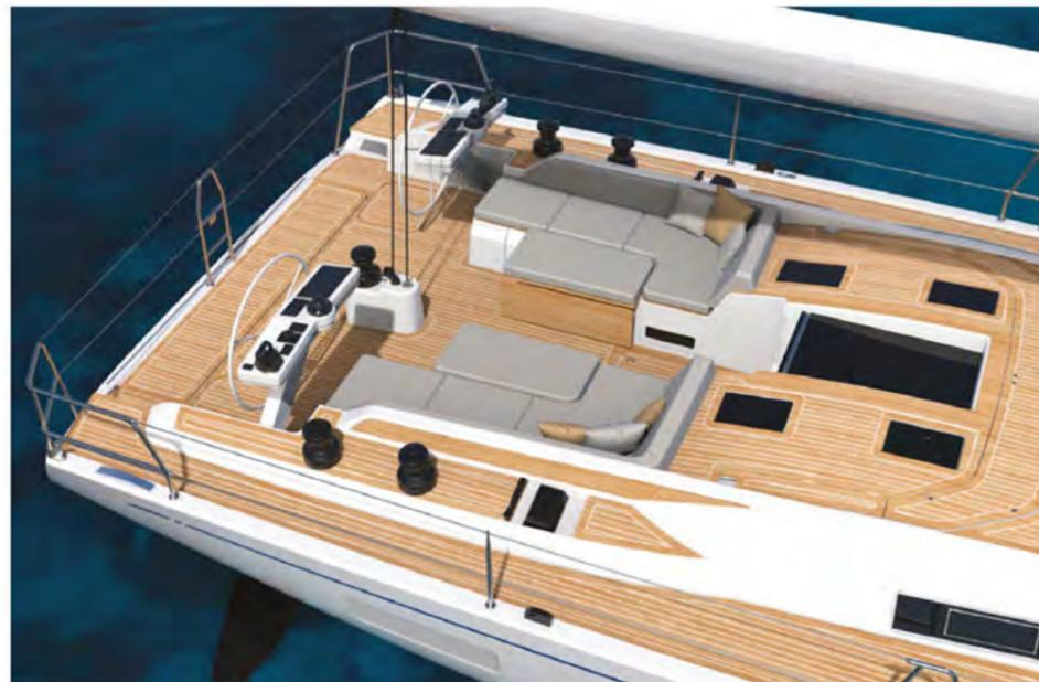
The five winches are electrically powered as standard, and equal size to allow functional redundancy and cross-sheeting. The main sheet can be on a captive winch as an option
